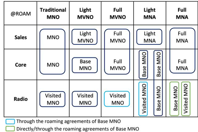
**Figure 3: Roaming operations for the different types of mobile operators.**
