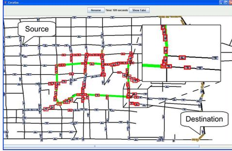
FIGURE 1: A simple VFN topology in downtown Chicago. The thicker, lighter shaded roads represent the virtual path over which messages are ferried, and the vehicles with dark borders are participating in the VFN.
